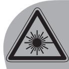
Laser Radiation. Do not stare into beam. Class 2 laser product
