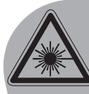
Laser Radiation. Do not stare into beam. Class 2 laser product
